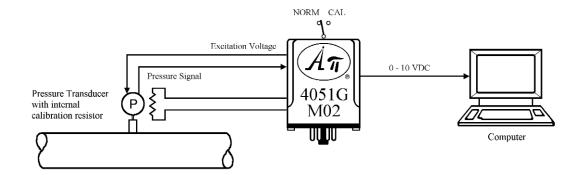
The API 4051 G M02 utilizes the pressure transducer's internal calibration resistor to unbalance the bridge to a specified value when the test switch is in the CAL position, ensuring accurate system calibration.
