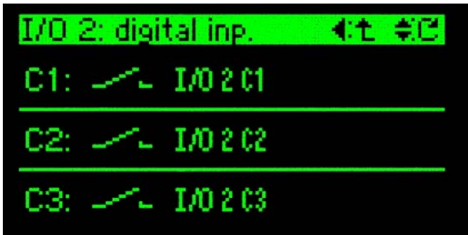
For each channel of digital input or output modules the output value and the channel text is displayed.
